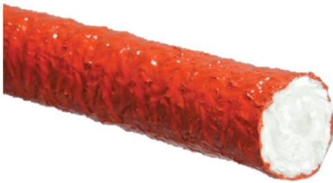
Pyrotex SG Rope is manufactured by Atlantex to provide efficient gasketing and sealing in high temperature applications, especially in environments where molten splash and flames are present. Pyrotex SG Rope is produced by coating high-density round fiberglass rope with a heavy layer of self-extinguishing silicone polymer.
